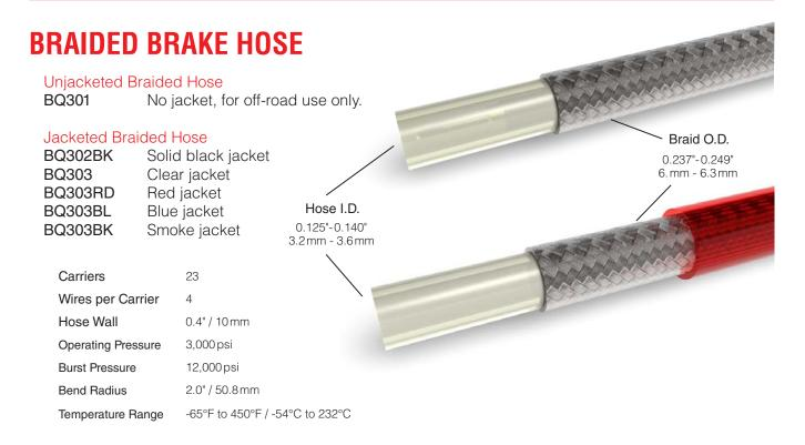
Compatible with DOT 3, 4, 5 (silicone-based), and 5.1 brake fluids, plus oil and most fluids. Warning: no gases or acids should be used.
